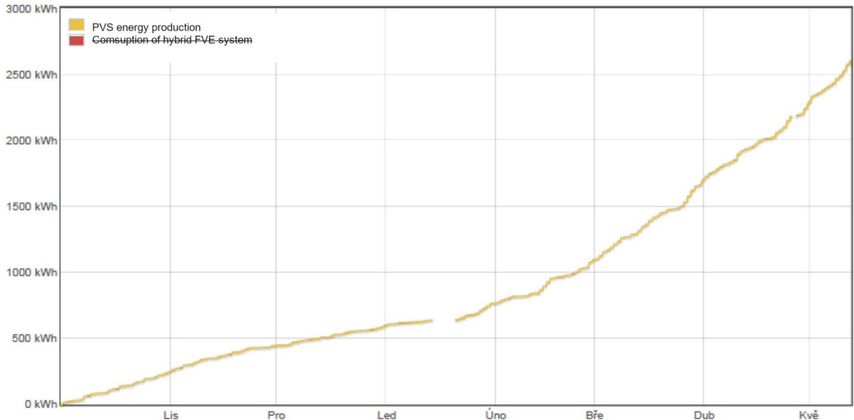
**The PV system produced 2 507 kWh in the 2016/17 heating season, i.e. 12.5% of total energy consumption, and in 2017/18 it was 3 500 kWh, i.e. 17.5% of total consumption!**
