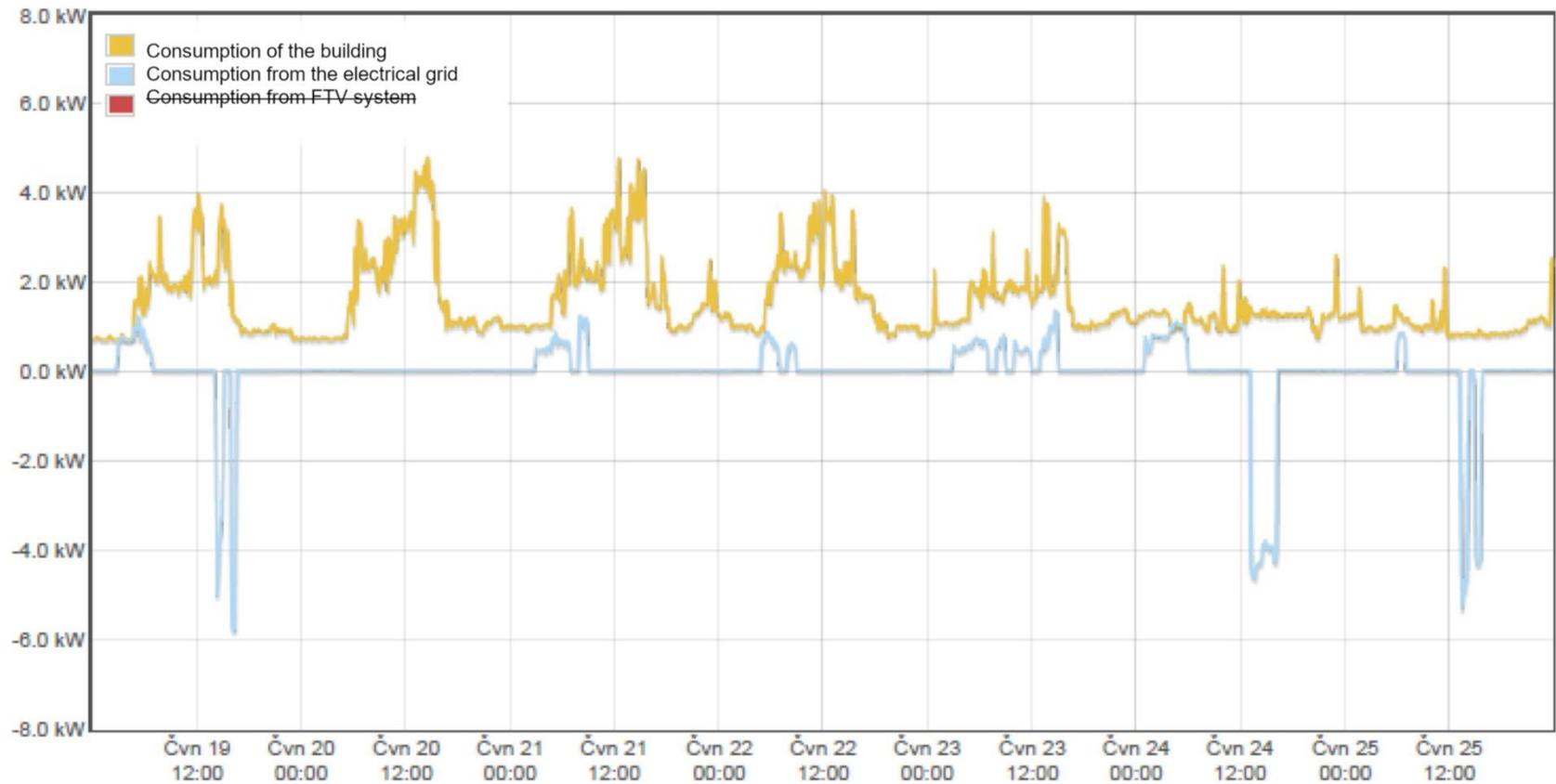
**Comparison of the real consumption of the building with the consumption from the grid - shows that low, controlled consumption takes place during the night while controlled supply occurs during the day (High Tariff)**
