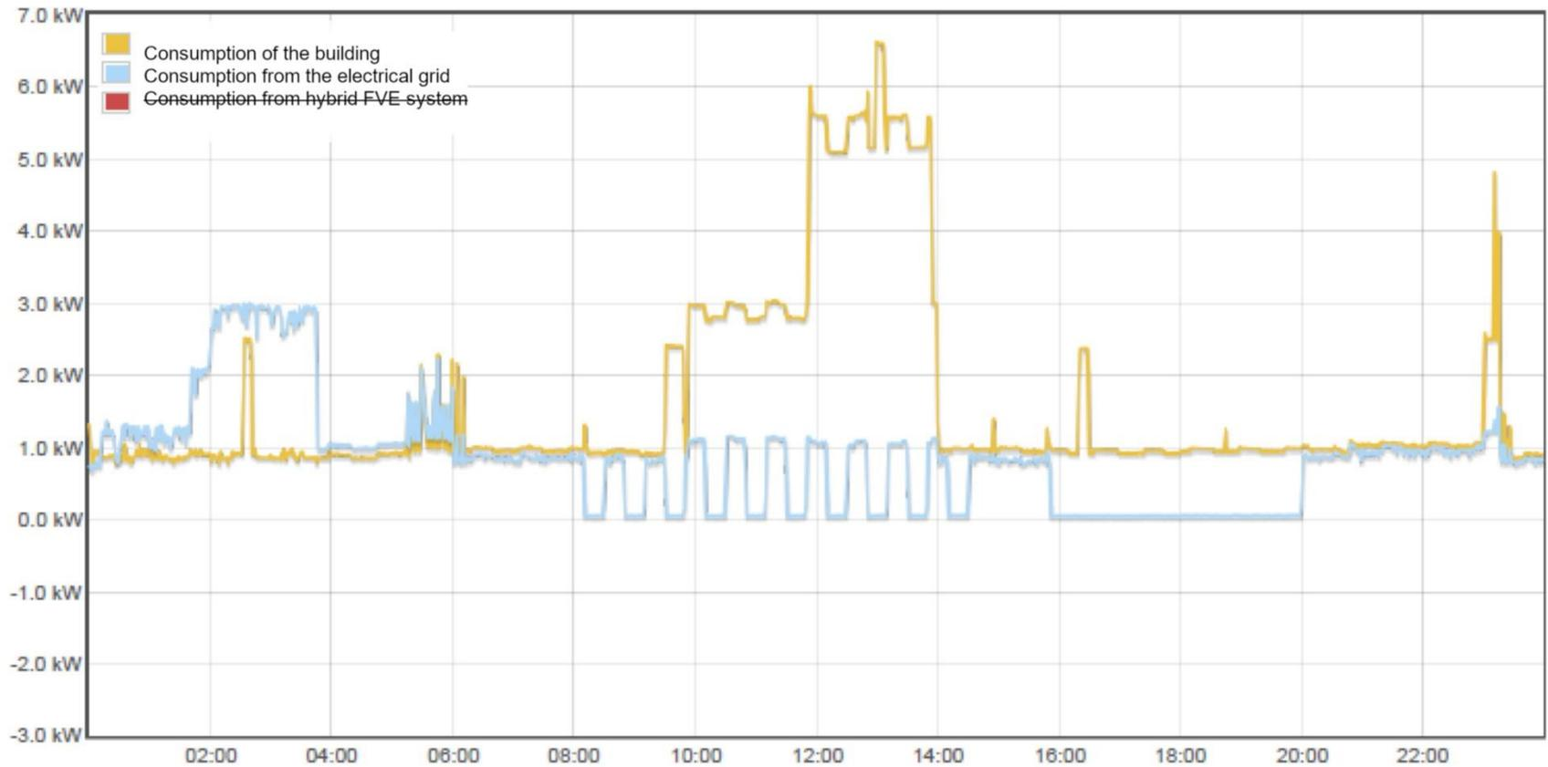
Regular off-grid mode (30 min intervals) when load increases (up to 6kW)
