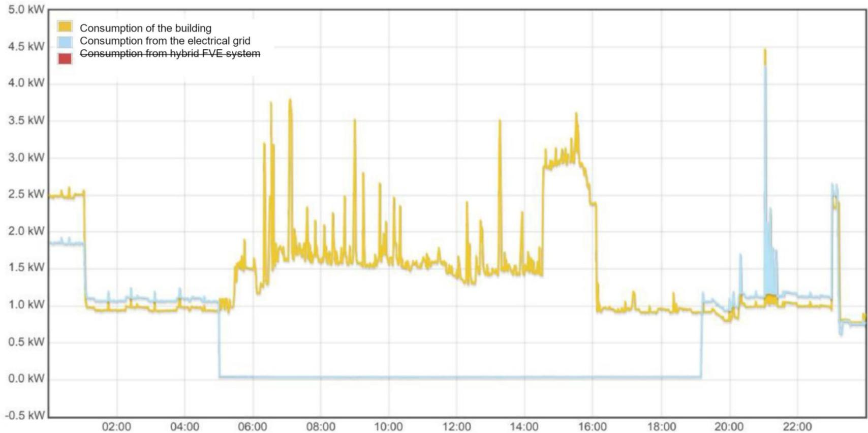
18.5. – experiment: zero consumption from 5 a.m. (maintained for 14 hours till 7 p.m.)
