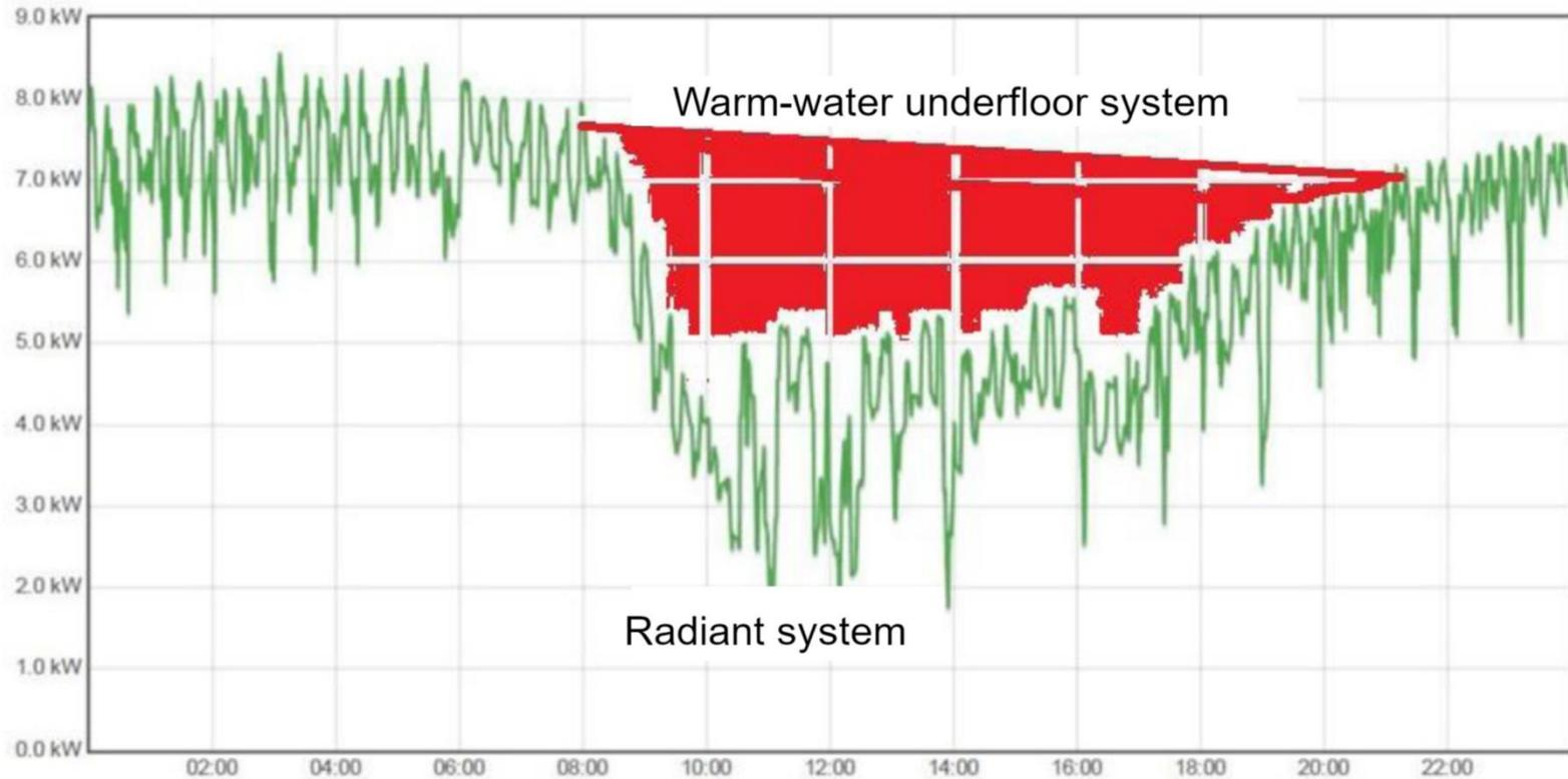
**The energy consumed for heating (by the radiant heating system) reacts flexibly to the change in outdoor temperatures and particularly to random heat gains (people – equipment) In contrast, a warm-water system with its great inertia and slow reaction speed is not capable of reacting quickly, which results in significant energy losses**
