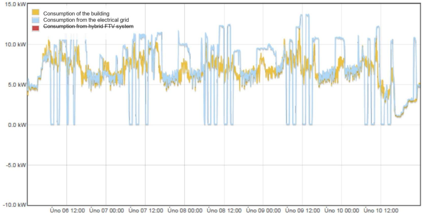
**Comparison of the real consumption of the building with consumption from the grid, showing the ability of the battery storage system to achieve zero consumption from the grid during peak periods (high tariff) and harmonize the consumption of the building over 24 hours.**
