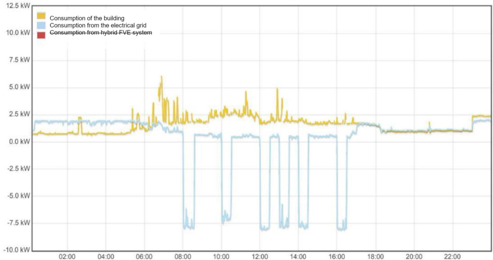
21.5.2018 - even consumption with controlled energy supply to the grid
