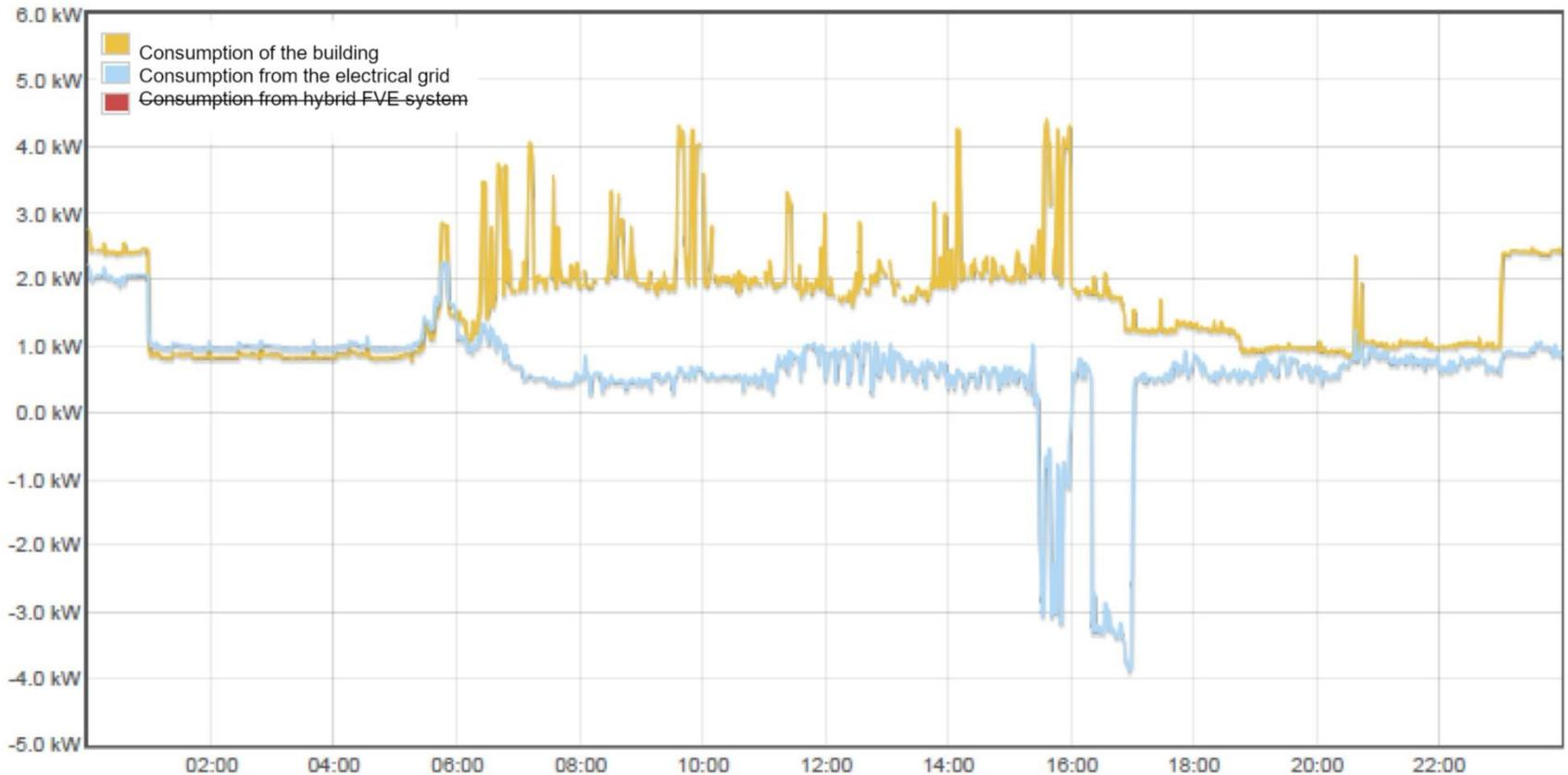
Maintenance of the daily power supply from the grid at a level below 1kW, with possible controlled overflow in the case of PVS overproduction
