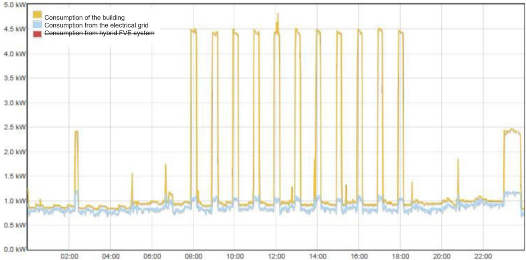
Maintenance of even consumption from the grid despite a load increase of 4.5 kW at regular intervals
