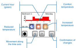
When you have finished, press the "**OK**" button and you will move to the program alteration option for the remaining days/day.
