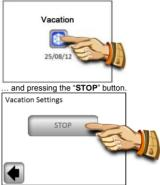
Note: In the "At Home" mode, the main screen is displayed enabling access to all functions, supplemented by a "Holiday" symbol with the date of return. You can stop the mode earlier by pressing the symbol, and then pressing the displayed "STOP" button.
