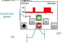
The control on the V25 receiver enables it to be set directly (On/Off, Timer 2Hours) and it takes precedence over the instructions of the central unit.
