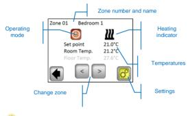
By pressing the "**Operating mode**" icon, you will have direct access to the settings of the parameters of the mode.
