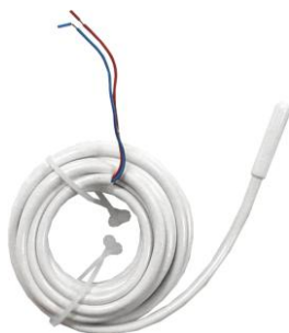
External sensor NTC type 10k \Omega at 25°C ( B = 3950 )
